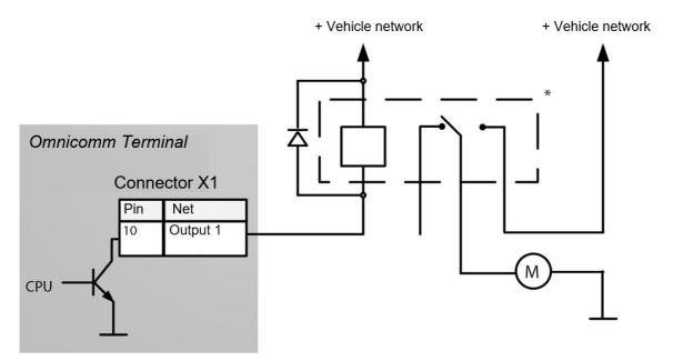
\* Relay with operation voltage suitable for the voltage of this vehicle network (12 or 24 VDC)
