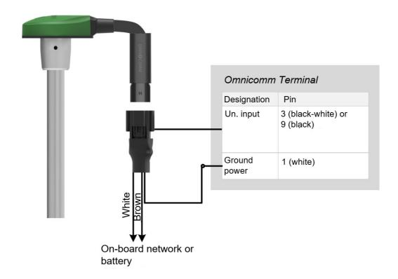
Connect several Omnicomm LLS-AF sensors to the Light terminal one by one, starting with 1 universal input.
