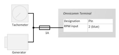
The place of connection to the tachometer shall be the point in the vehicle electric network, in which the pulse signal frequency is proportional to the engine RPM.
