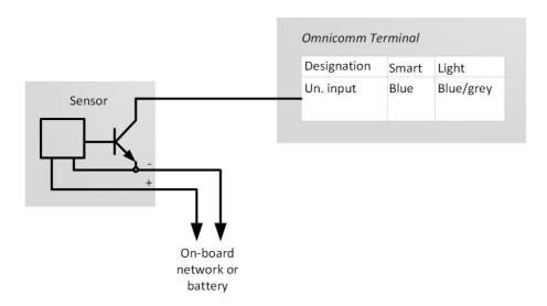
Connect contact sensor according to the diagram:
