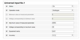
"Minimum value of measured parameter" – set the minimum value to be measured by the sensor (in the units of measurement of this value).
