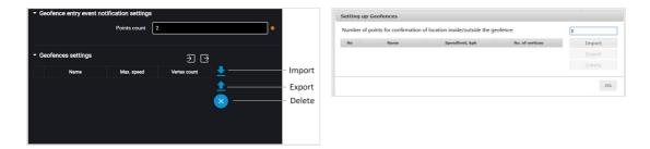
"Number of points to confirm being inside/outside the geofence" – specify the number of successively defined vehicle coordinates required to register the vehicle being inside or outside the geofence. Coordinates determination period – 1 sec. Possible values: from 1 to 10.
