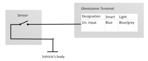
As the contact sensor you can use standard elements of equipment control (activation buttons / limit switches / sensors triggered by excess pressure or temperature, etc.) or an additionally mounted sensor. We recommend that you first look for possibility of connection to a standard device and install an additional sensor only if there is none.
