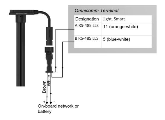
Connect Omnicomm LLS-AF fuel level sensor according to the diagram:
