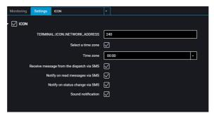
"ICON" – check the box to display the data from the terminal on the Omnicomm ICON display
