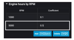
Enter the RPM value in the "Revolutions per minute" field, in "Coefficient" field enter the value of conversion factor to calculate engine hours.
