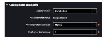
"Accelerometer" – enable/disable the use of accelerometer for measuring the vehicle acceleration.
