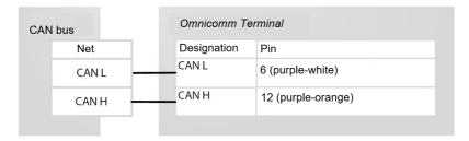
Configuring the reception of data on the fuel volume in the tank from the vehicle CAN bus Connect and configure reception of the vehicle equipment operation parameters from CAN J1939 data bus and set the setting of fuel sensor – "CAN Sensor".
